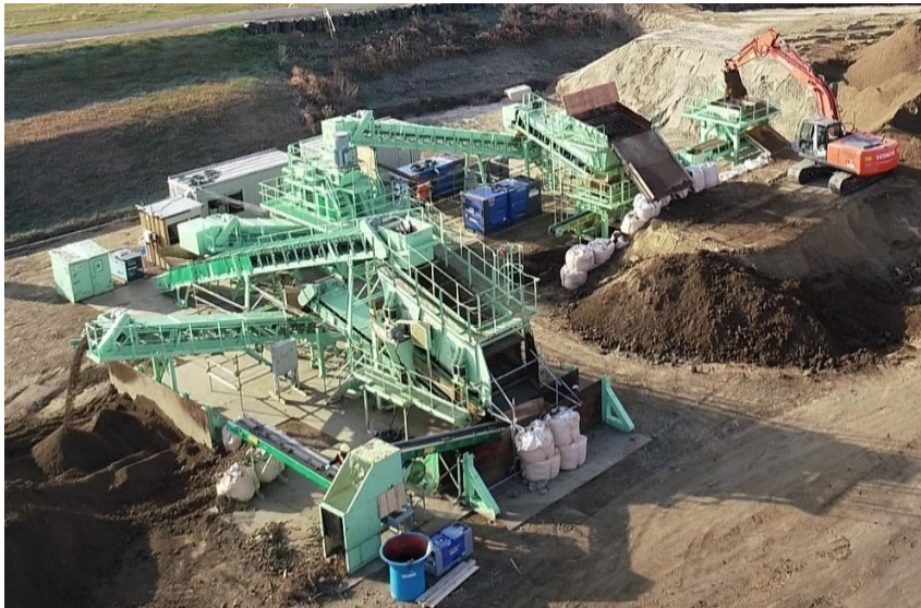
Rotary Crushing and Mixing Method (a.k.a. Twister®)
